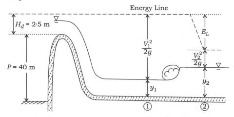
The figure shows an overflow spillway which is 40 m high. At the design energy head of 2.5 m over the spillway, determine—
